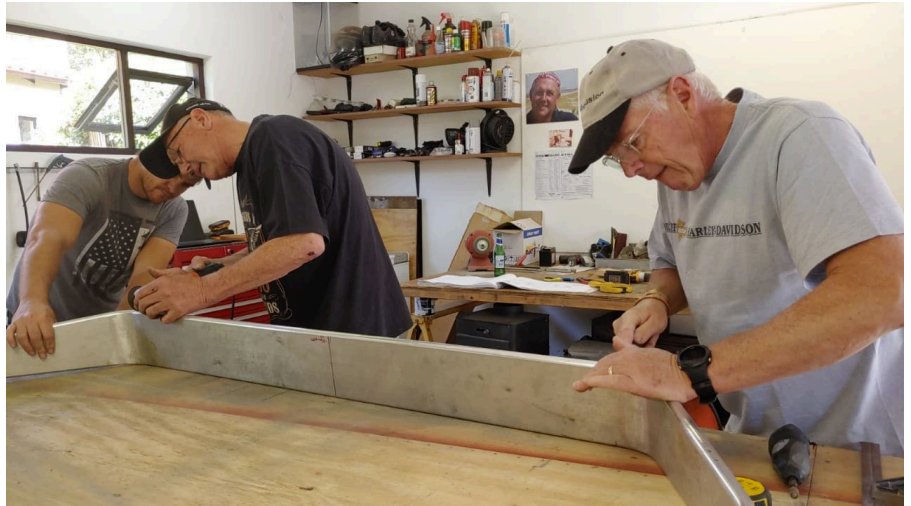
Slowly filing away material to make sure the slots weren't oversized
