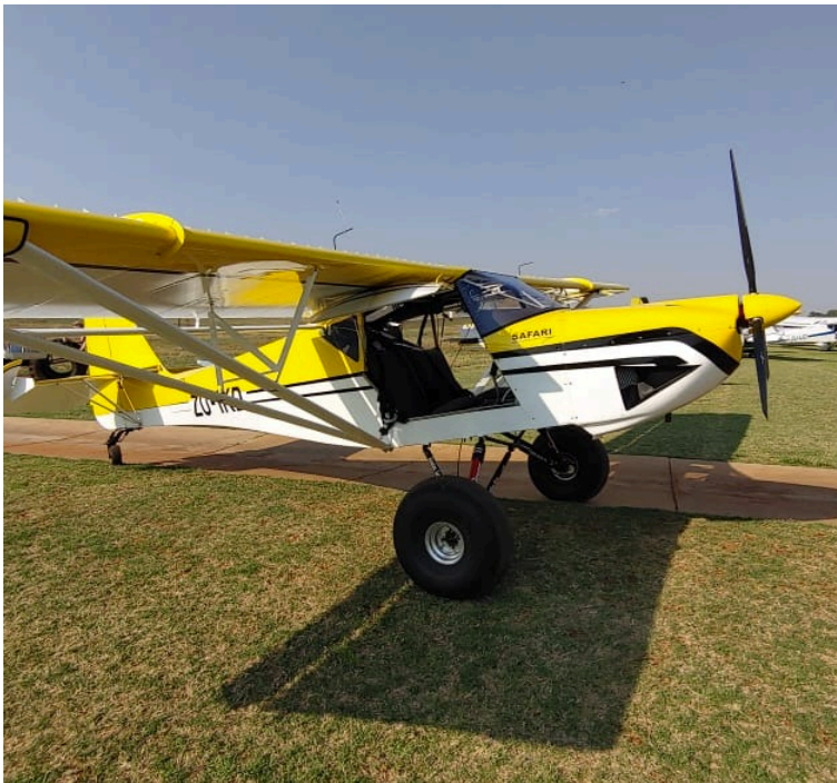
KFA Safari - Alaskan Landing Gear and Rotax 915
