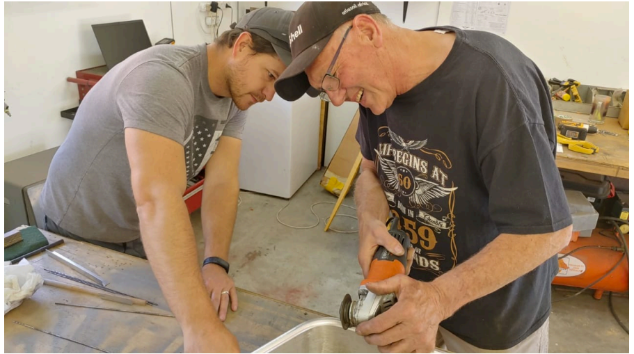
Rob and Ant grinding the slots to fit the mounting bolts on the undercarriage
