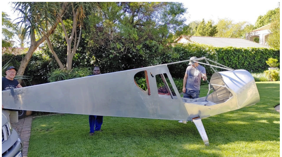
Finally she's on her legs! The nose wheel is also ready to be fitted – it mounts onto the firewall
