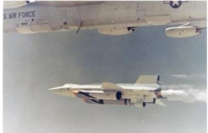
*An ablative coating to protect the craft from the high temperatures was added. The X-15 was then covered with a white sealant coat and mounted with additional external fuel tanks giving it an extra 60 seconds flight*
