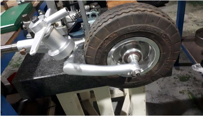
*Scratch built tailwheel assembly*
