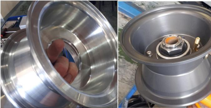
*Main wheel rims after machining, before and after anodising*
