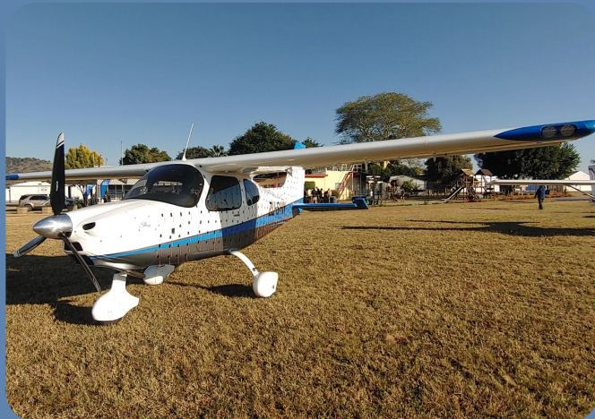
The new HW Sling complete with aero flow "tassles" for spin testing
