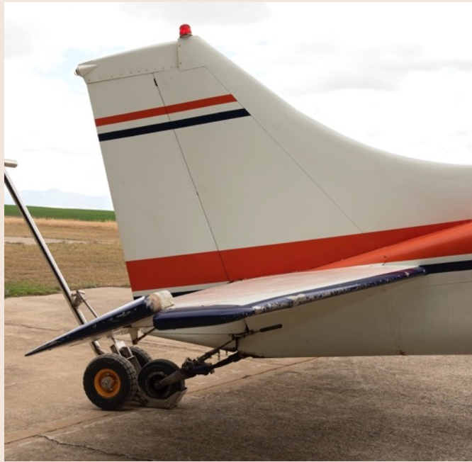
The empennage comes from a Cessna 170
