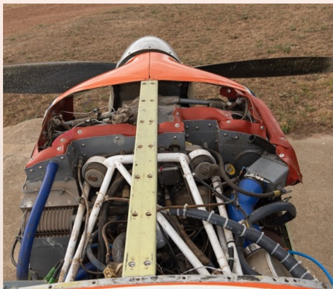
The Vansin uses a Twin Comanche 160hp engine
