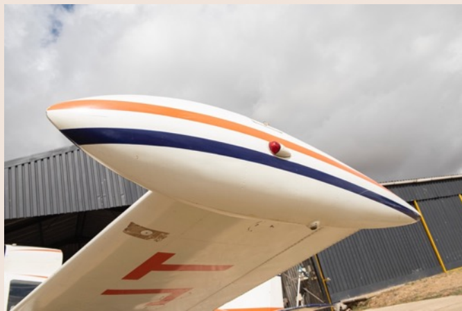
Tip tanks come from a Twin Comanche – which also supplied the engine and original cowling
