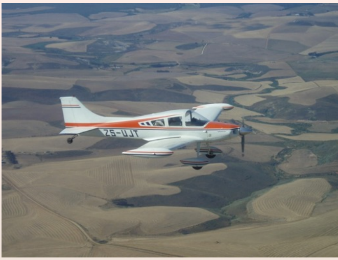
The Vansin in 2003 - before it had its nose stretched to move the CoG forward
