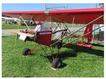
**The Legal Eagle XL** Single seat, handles a 275 lbs (125 kg) pilot. Wingspan is 32" longer, 246 lbs empty weight. One man wing removal. Better Half VW 30 hp engine
