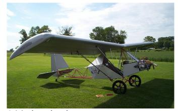
**Original Legal Eagle** Single seat, designed for pilot up to 220 lbs (100 kg) 6' tall (1,83M). Designed around the Better Half VW 30 hp engine. Two-person wing removal for storage. 244 lbs empty weight
